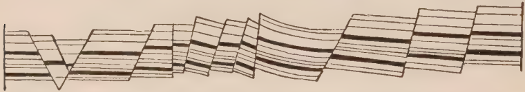
FIG. 254. — Section across Yarrow Colliery, England, illustrating the law of normal faults. The surface is restored. (After De la Beche.)
